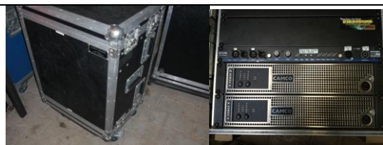
Seeburg acoustic Line, Camco D2+PL-Audio D14k2: Amprack+1x Controller DBX Driverack 260 Technische Daten: 2x1000W, 2x2000W
